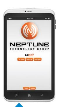
From here the user can select one of the three different functions of the app – RF Test, Data Log, or Off Cycle.
