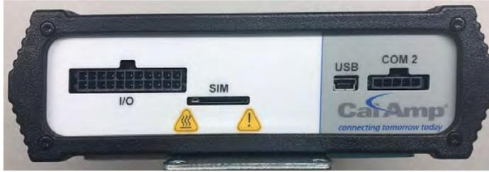
Figure 95 – Modem Back View
