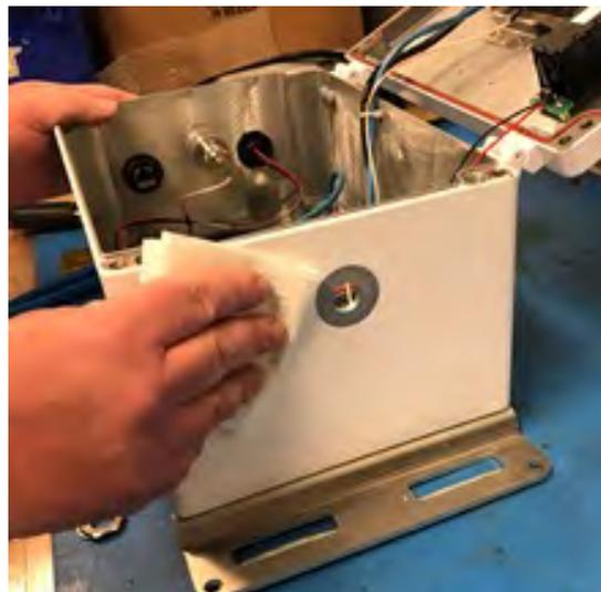
Figure 119 – Clean Antenna Mounting Area
