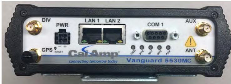
Figure 104 – Cellular Modem Front - Status LEDs
