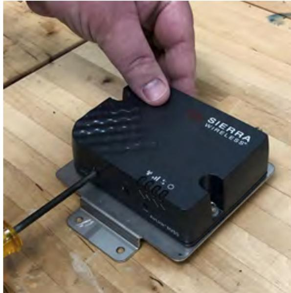
Figure 114 – Remove SIM Card
