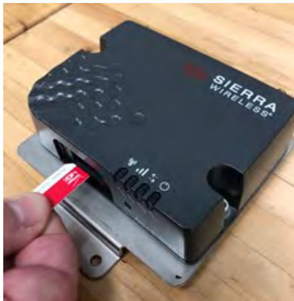
Figure 115 – Insert New SIM Card
