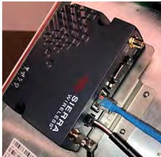
Figure 117 – Reconnect Cables to Sierra Modem
