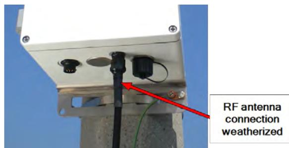
Figure 65 – Weatherized RF Port
