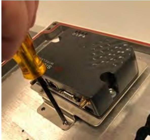
Figure 116 – Mount Sierra Modem on Gateway Door Panel
