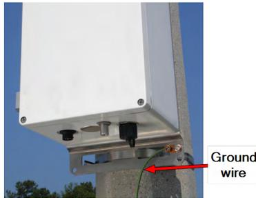
Figure 63 – Attach Ground Wire
