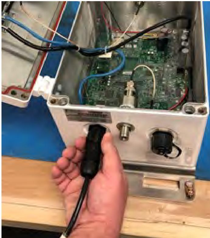
Figure 111 – Disconnect Power to Collector
