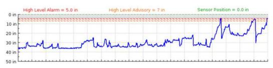
buildup, grit accumulation, roots, or pipe degradation, the software detects the irregular trends and sends advisory notifications. When conditions reach a threshold setting, an email is automatically issued with a screenshot from the SmartTrend report, and the green circle icon turns to an orange circle on the site map.
