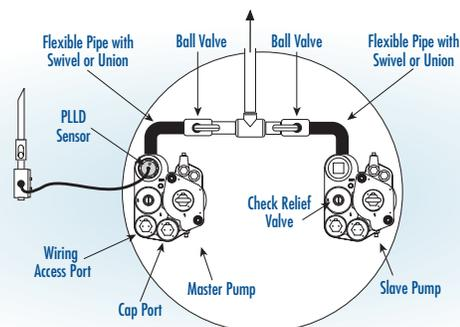
Manifolded systems provide up to 2X the flow rate and improved uptime. Manifolded systems can be configured in sumps 42" in diameter or greater.
